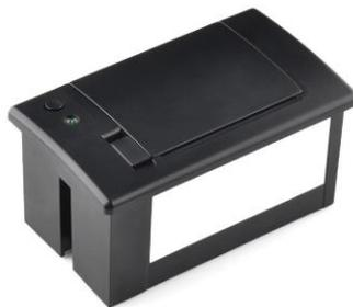
*Printer without case* (Xiamen Cashino Electronic Technology Co., Ltd. Model KP-628C – <http://www.csntek.com>). This is an OEM printer with **cutter**. Paper size is 58 mm. You can purchase this printer in Aliexpress for about 40.00 EUR. This printer uses an external paper roll to increase paper capacity, and includes a **cutter** to ease voucher delivery.
